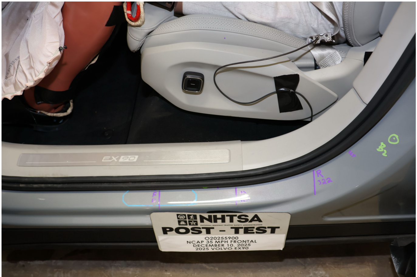
Photo No. 037 - Post-Test Driver's Seat Fore-Aft Markings
