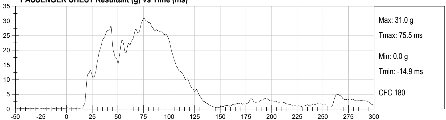
PASSENGER CHEST Resultant (g) vs Time (ms)
