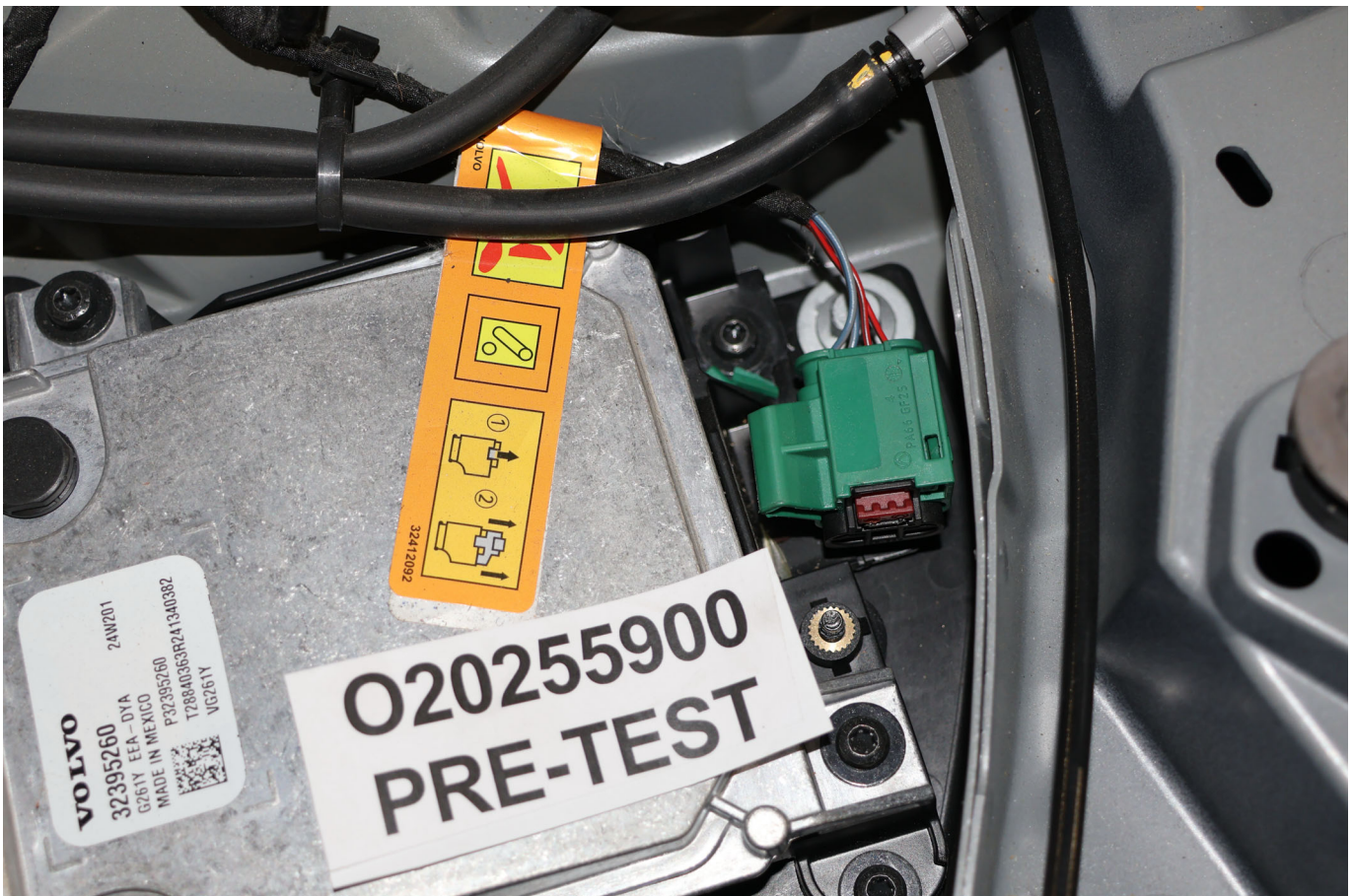
Photo No. 305-03 - First Responder Warning Label
