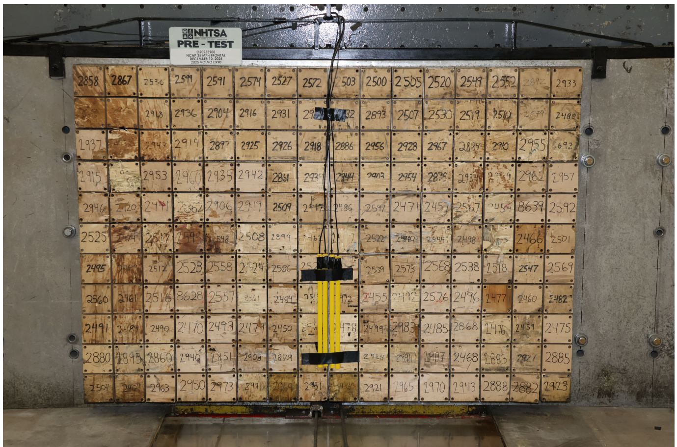
Photo No. 002 - Pre-Test Load Cell Wall
