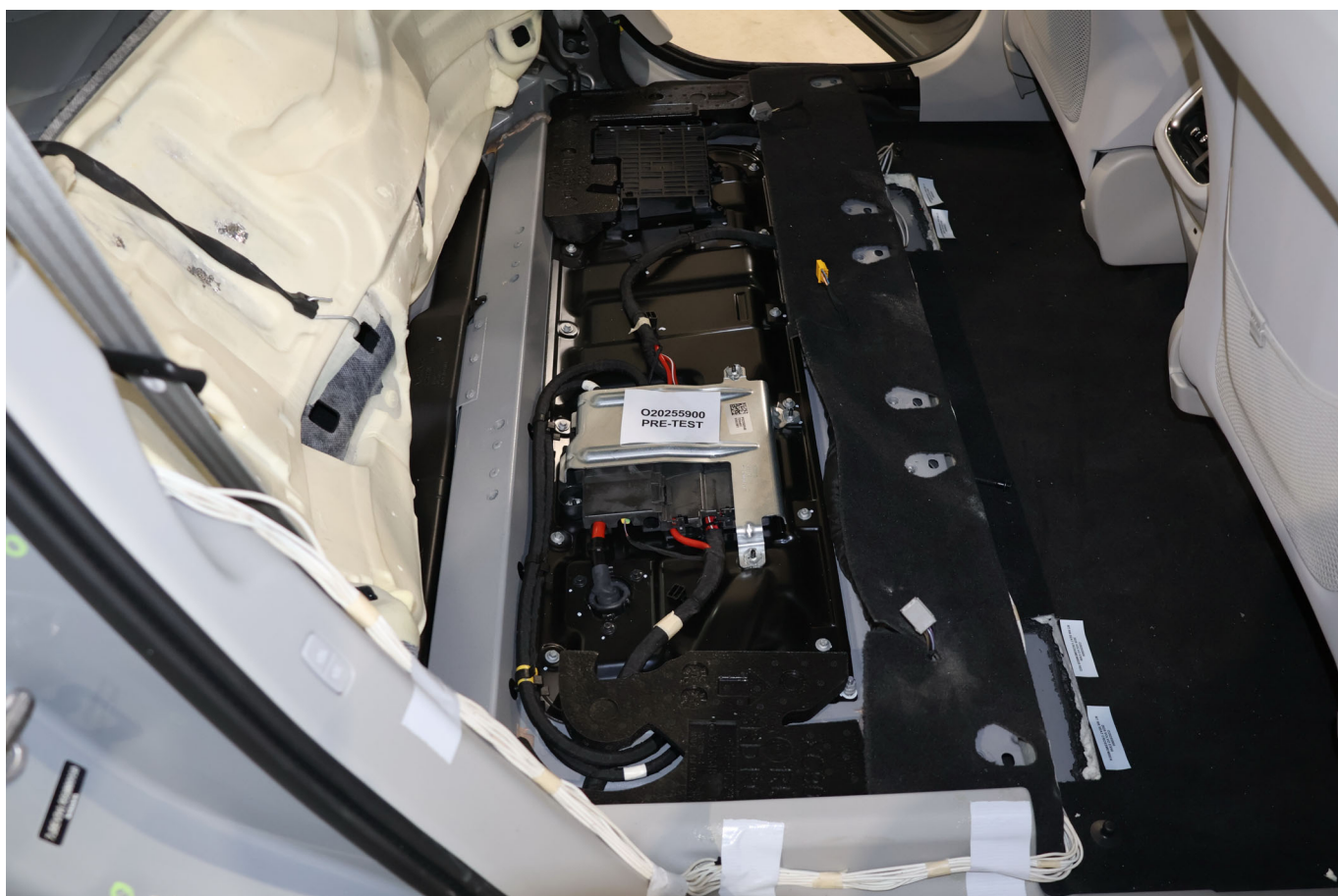
Photo No. 305-09 - Pre-Impact View of Propulsion Battery
