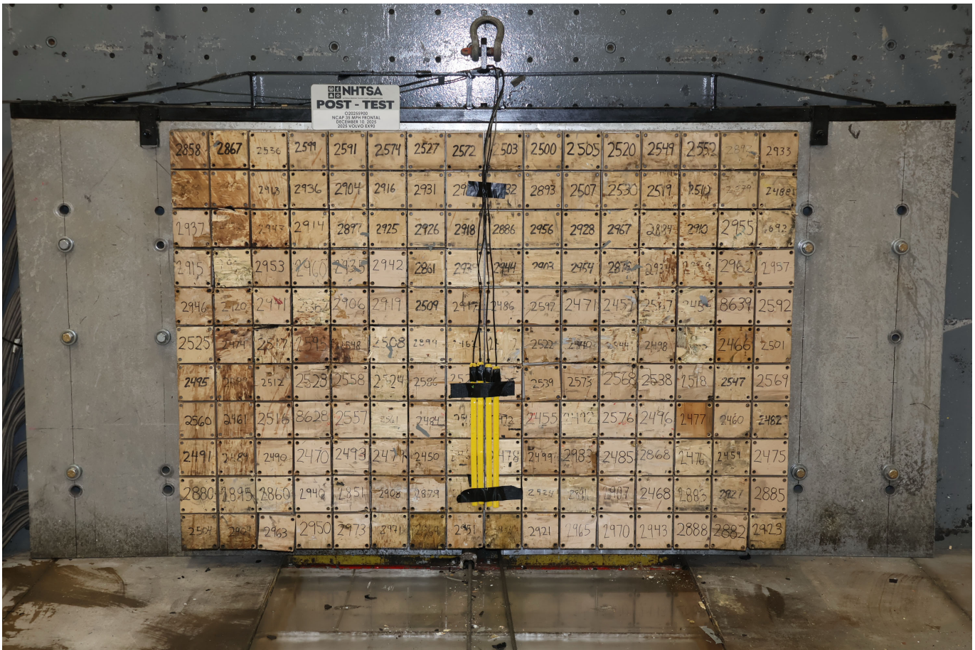
Photo No. 003 - Post-Test Load Cell Wall
