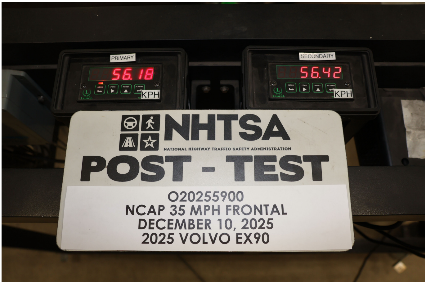
Photo No. 076 - Post-Test Speed Trap Read-Out
