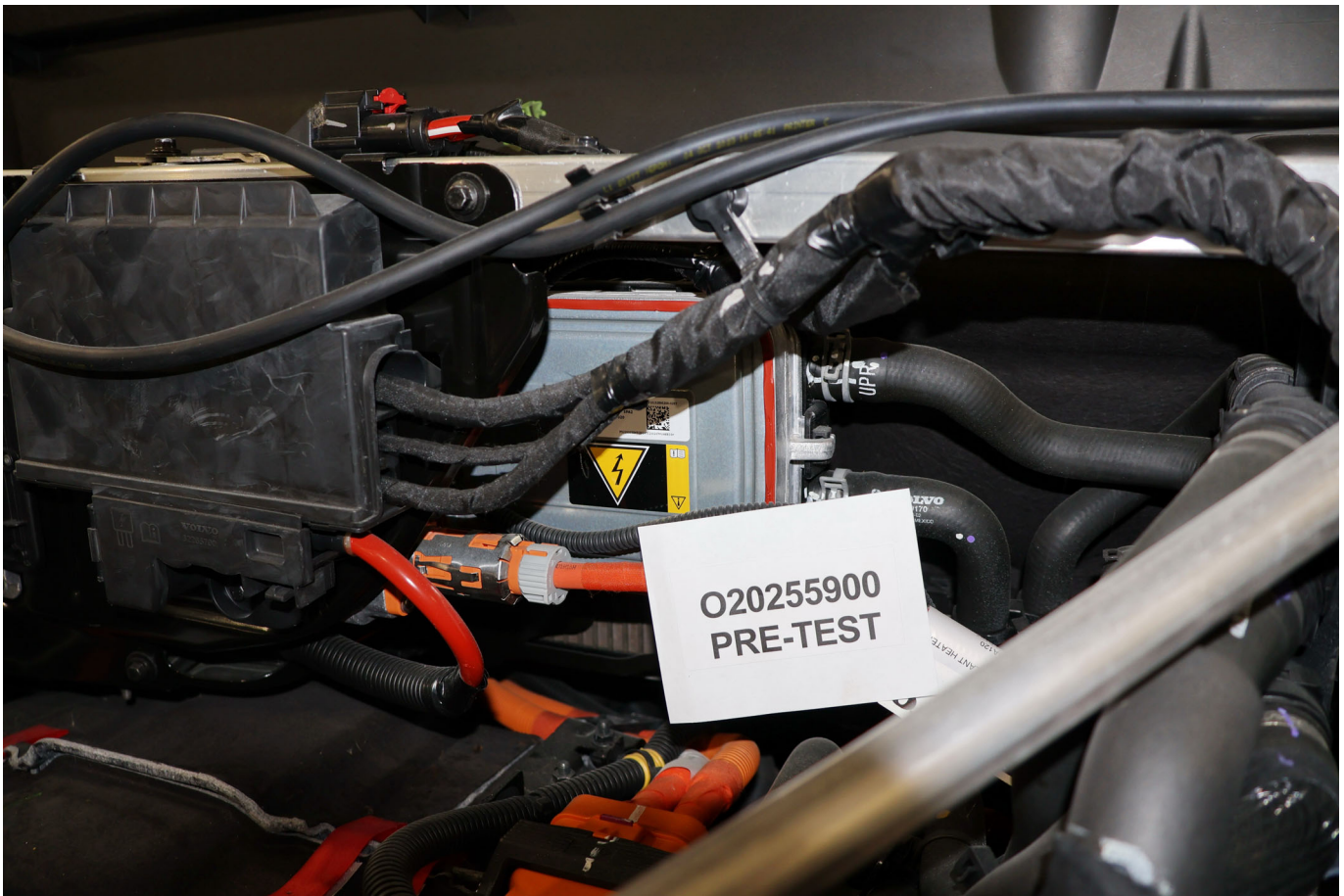
Photo No. 305-02 - Power Inverter Warning Label
